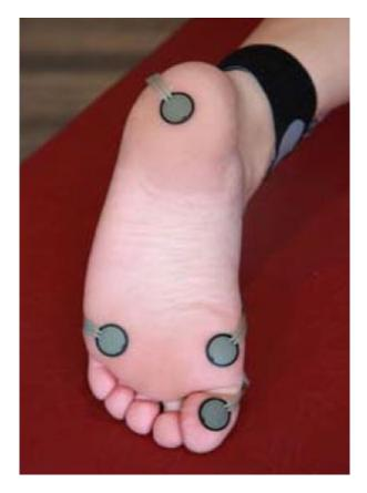
While four FSR sensing areas are available, the footswitches may be used with one to four FSR sensing areas.
